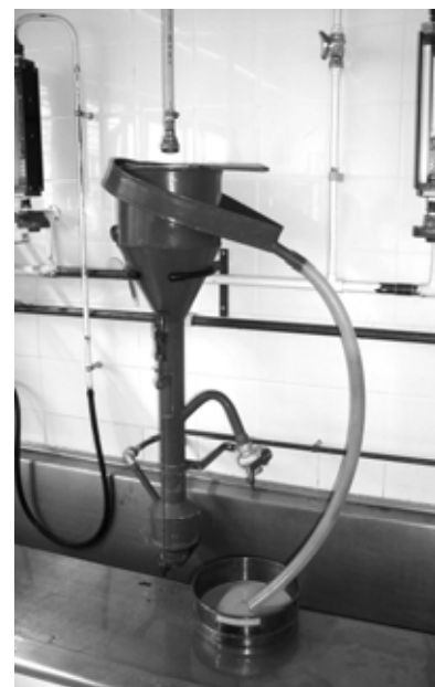
Figure 23 Seinhorst's extraction apparatus for the extraction of cysts from non-dried soil
