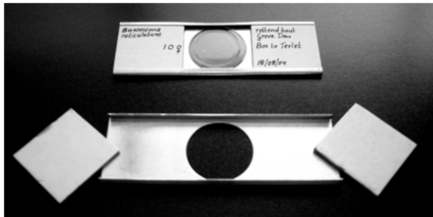
Figure 25. Prepared Cobb slide, and an aluminium holder with two cardboard pieces.
