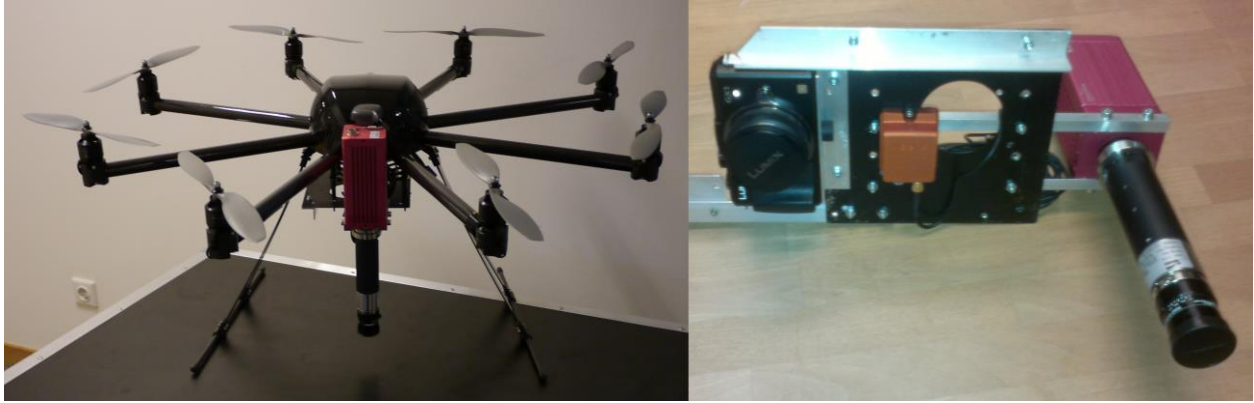
Fig. 2: The light-weight hyperspectral mapping system consisting of an Aerialtronics Altura AT8 octocopter (left) and the mapping system (right) composed of a Panasonic Lumix GX1 camera, XSens MTi-G-700 INS, and a pushbroom spectrometer.
