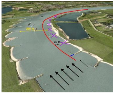
Location of training dam (red), intake weir (blue) and removed groynes (purple).
