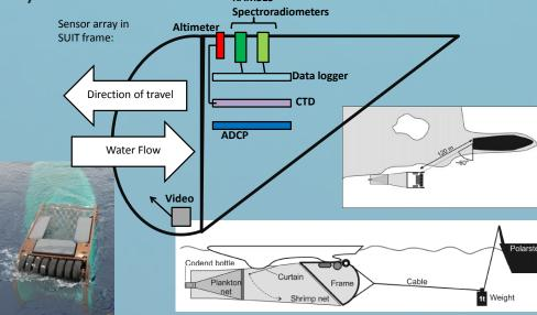
Above: the SUIT net samples the under ice surface water (2m) and is equipped with two parallel nets: a 7 mm half-mesh and a 0.3 mm mesh. Sensors are used to measure e.g. water temperature, depth, water flow and ice thickness.
