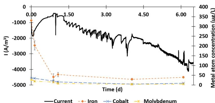
**Figure 2.** Current and catholyte concentrations of iron, cobalt and molybdenum during startup of an abiotic CO<sub>2</sub> fed reactor.
