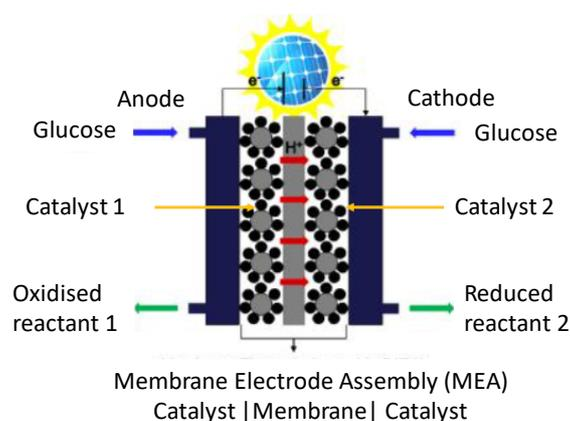
Figure 2. A paired electrolysis cell for the oxidation and reduction of glucose using high surface area electrodes (catalysts deposited on carbon support), separated by a membrane<sup>1</sup>.
