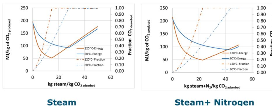
**Figure 1.** Energy required to desorb CO<sub>2</sub> from an adsorbent with 0.5 mmol/g capacity within a 100 mbar vacuum and final pressure CO<sub>2</sub> of 30 bar.
