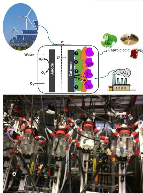
**Figure 1.** Schematic (top) and lab (bottom) setup of the microbial electrosynthesis system.
