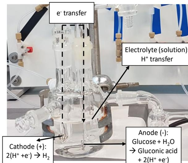
Figure 1. The electrocatalytic oxidation of glucose for the production of gluconic acid, balanced by hydrogen evolution (overall water reduction) using bulk electrodes.
