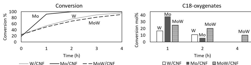
Figure 2. Stearic acid conversion over Mo/CNF, W/CNF and MoW/CNF (250 mg catalyst, 2 g stearic acid, 50 mL solvent, 30 bar H<sub>2</sub>, T = 350 °C).
