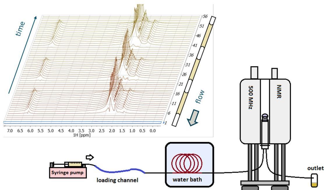
**Figure 1,** *Top*) NMR spectra collected over allow for a composition analysis of the reaction mixture. *Bottom*) the set-up: a slug flow of reactants is prepared in the loading channel and pushed through reactor and the NMR for in-line detection.
