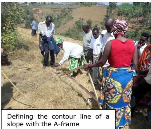
Defining the contour line of a slope with the A-frame
