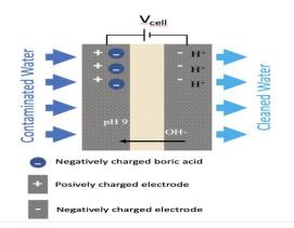
Fig. 1. Electrochemical removal of contaminants. Water is split into H<sup>+</sup> and OH<sup>-</sup> on the right-hand electrode. OH- migrates to the left side, increasing the pH. Acids, donate a H<sup>+</sup>, and become negatively charged, and are subsequently absorbed by the positively charged electrode.
