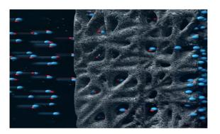
Impression of the carbon electrode where the contaminants are absorbed. An acid (blue with red balls) enters the high pH electrode and loses a H<sup>+</sup> (red ball). The remaining negatively charged acid (blue ball) sticks to the positively charged electrode.
