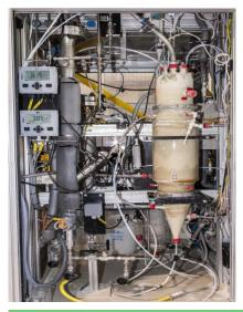
Sulfur formation in the second reactor vessel of the the Thiopaq O&G Ultra pilot plant at ETE.
