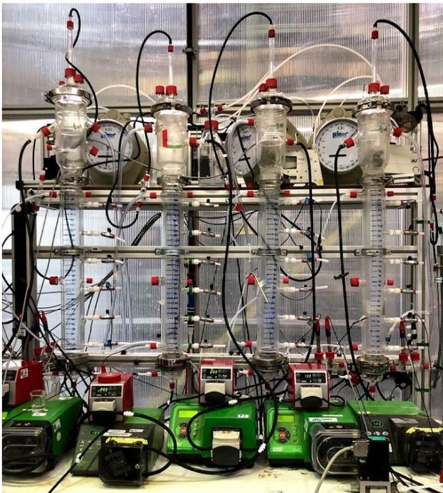
Figure 1 Lab-scale UASB reactors
