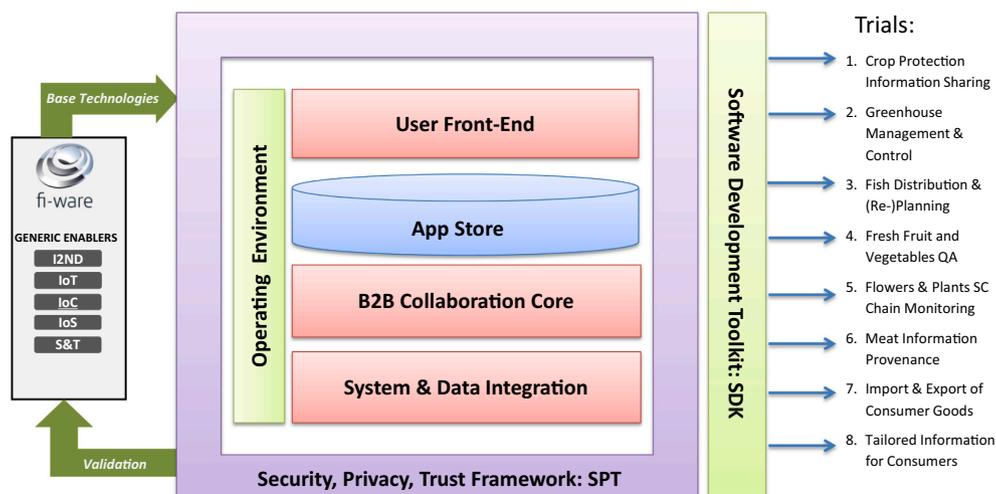
Fig. 5. The FIspace platform architecture built on FIWARE GEs the left) and the eight trials (Kruize et al., 2014).
